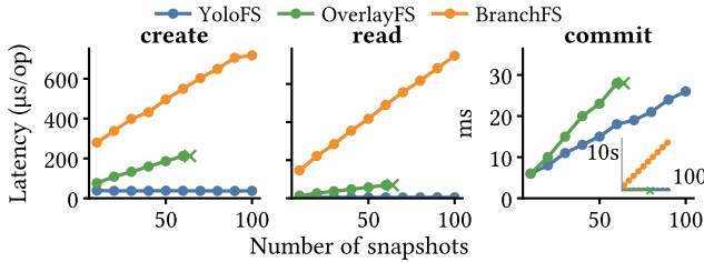
Figure 10. Snapshot scalability. As the number of snapshots grows, do filesystems become slower? (OverlayFS fails at ~50 snapshots.)
